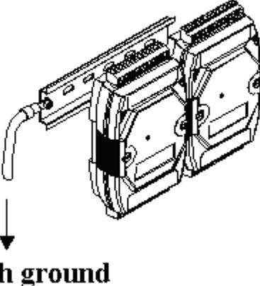
The diagram shows two DRS-125 modules mounted on a DIN rail. A wire is connected to the rail and labeled "to earth ground".
