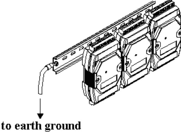
The diagram shows three DRS-240 modules mounted on a DIN rail. A wire is connected to the rail and labeled "to earth ground".
