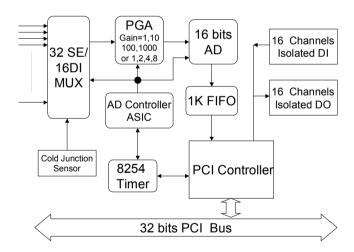
Figure 1. PCI-1114(A) Fundamental function block
