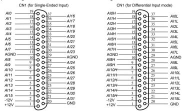
Figure 4. Pin Assignment of CN1
