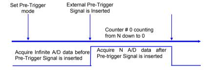
If the application acquires data after the pre-trigger signal, only the last N data needs to be stored. The maximum value of N is 65535. If the application only needs to acquire data before the pre-trigger signal, set N=1. Only one extra data will be sampled after the pre-trigger signal.
