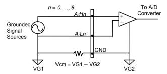
Figure 8. Grounded source and differential input
