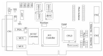
Figure 2. PCB Layout of PCI-9114 Rev. B1
