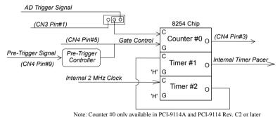
Figure 16. Timer/Counter system of PCI-9114(A).
