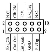
Figure 6. Figure 2.3 Pin Assignment of CN4
