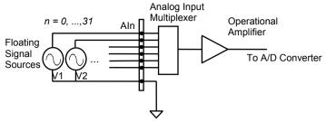
Figure 7. Signal sources and single-ended connection
