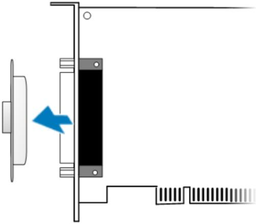
Step 7: Remove the connector cover from the PCI-822/826 Series card.
