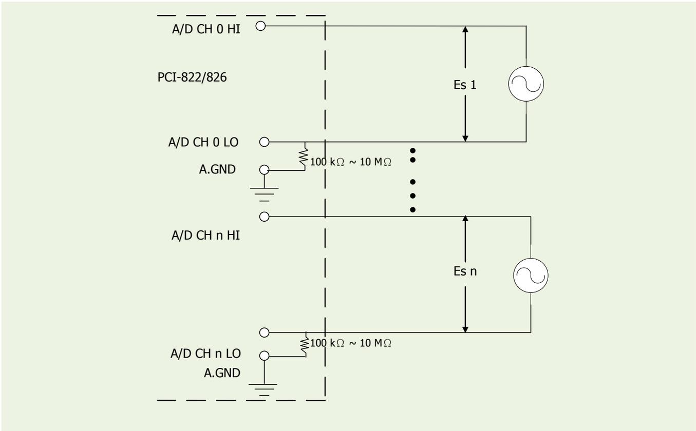
**Figure 2.5-6: Connecting to a 4 ~ 20 mA Source**
