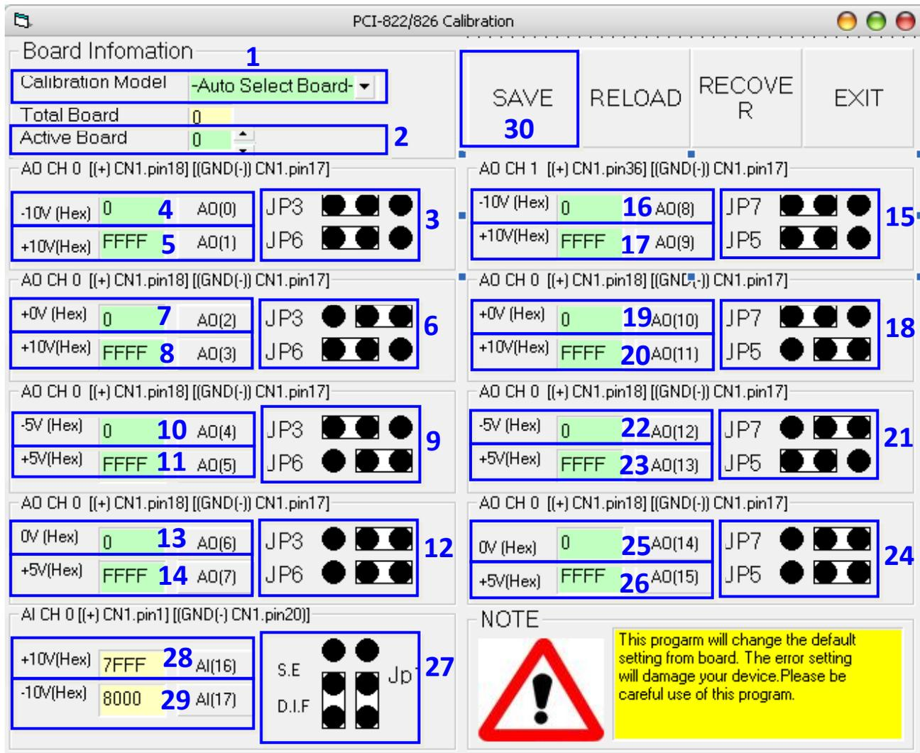
The following pin assignments are used in the calibration process.
