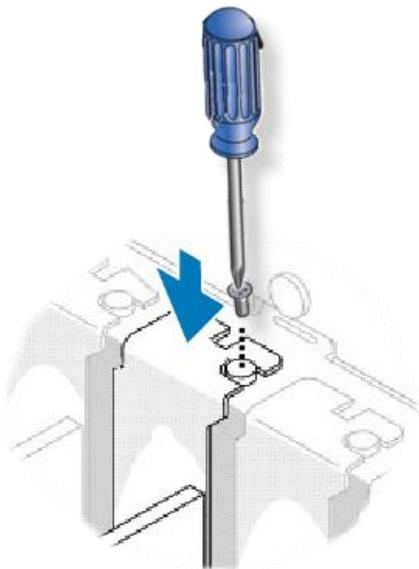
Step 9: Secure the PCI-822/826 Series card in place using the retaining screw that was removed in step 5.
