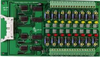
The DB-16P is a 16-channel isolated Digital Input daughterboard with optically isolated inputs that consist of a bi-directional optocoupler with a resistor to allow current sensing. The DB-16P can be used to sense DC signals from TTL levels up to 24 V, or can be used to sense a wide range of AC signals. This board can also be used to isolate the Host system from high common-mode voltages, ground loops and transient voltage spikes that can often occur in harsh industrial environments.
