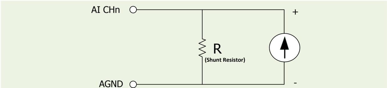
**Example:** A 20 mA source current through a 125 Ω resistor (e.g. 125 Ω, 0.1% DIP Resistors) between + and – terminals and the board will read a 2.5 V<sub>DC</sub> voltage. You can use the  $I = V/R$  (Ohm’s law) to calculate what value the source current should have.
