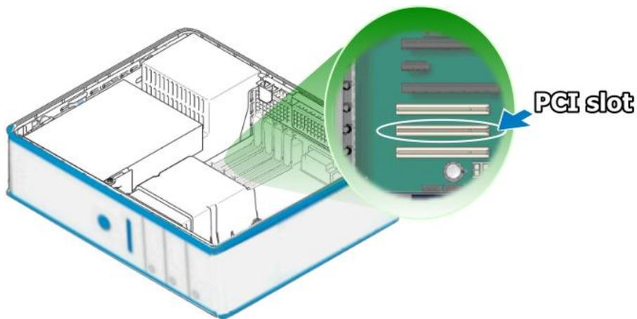
Step 6: Remove the screw holding the cover for the PCI slot in place and then remove the slot cover from the PC. Ensure that you do not misplace the screw.
