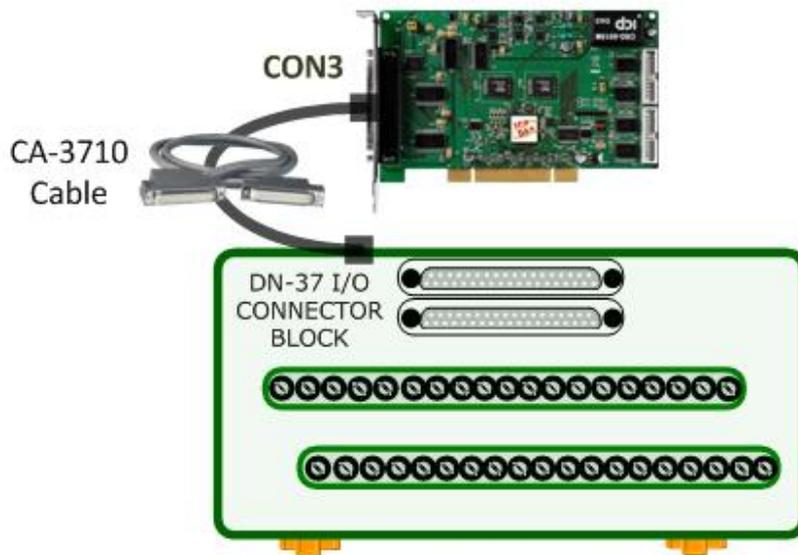
**Step 2:** Set the JP1 jumper (Analog Input Type) on the PCI-822/826 Series card to **Single-ended** mode (see [Section 2.2.1](#) for more details), and then **connect the AOO\_Out (Pin18) to the AIO (Pin1)**, and **connect the A.GND pin (Pin17) to the A.GND pin (Pin17)**.
